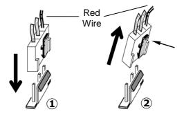
You should ensure that connector is inserted correctly so that the red wire is towards the top of the terminal.
