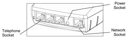
The base unit has 5 sockets for connections: TEL ( $\cong$ ) IN, COM0 (not used), COM1 (not used), POWER ( $\not\leftarrow$ ), and finally NETWORK ( $\searrow$ ).
