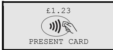
In order to perform a contactless transaction you must type in the transaction amount from the idle screen on your terminal.
